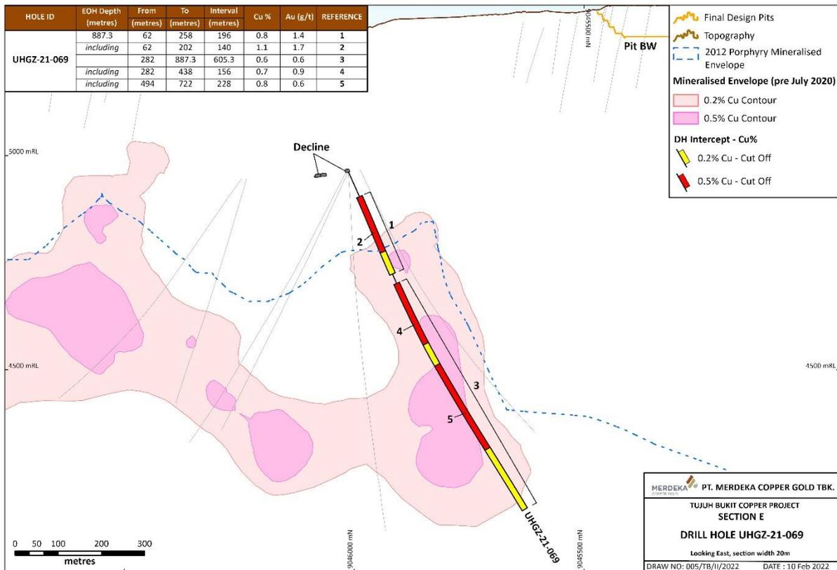
Figure 6: Drill section E, showing drill hole UHGZ-21-069 along with open mineralised envelopes at depth and drilling intercept information.
