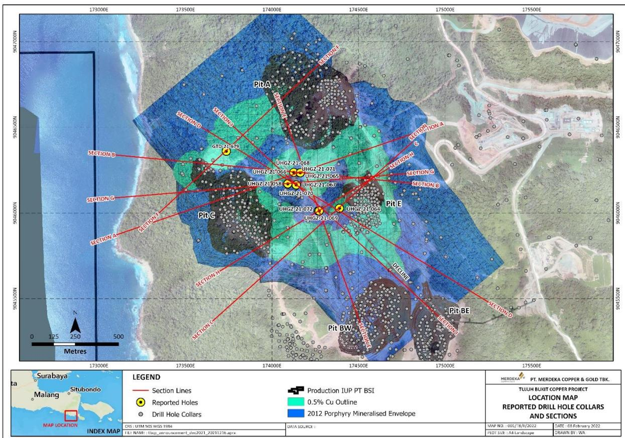
Figure 1: Location map of Tujuh Bukit Copper Project showing reported drill hole collars and sections, 2012 Mineralised outline, 0.5% copper contour and surface features.
