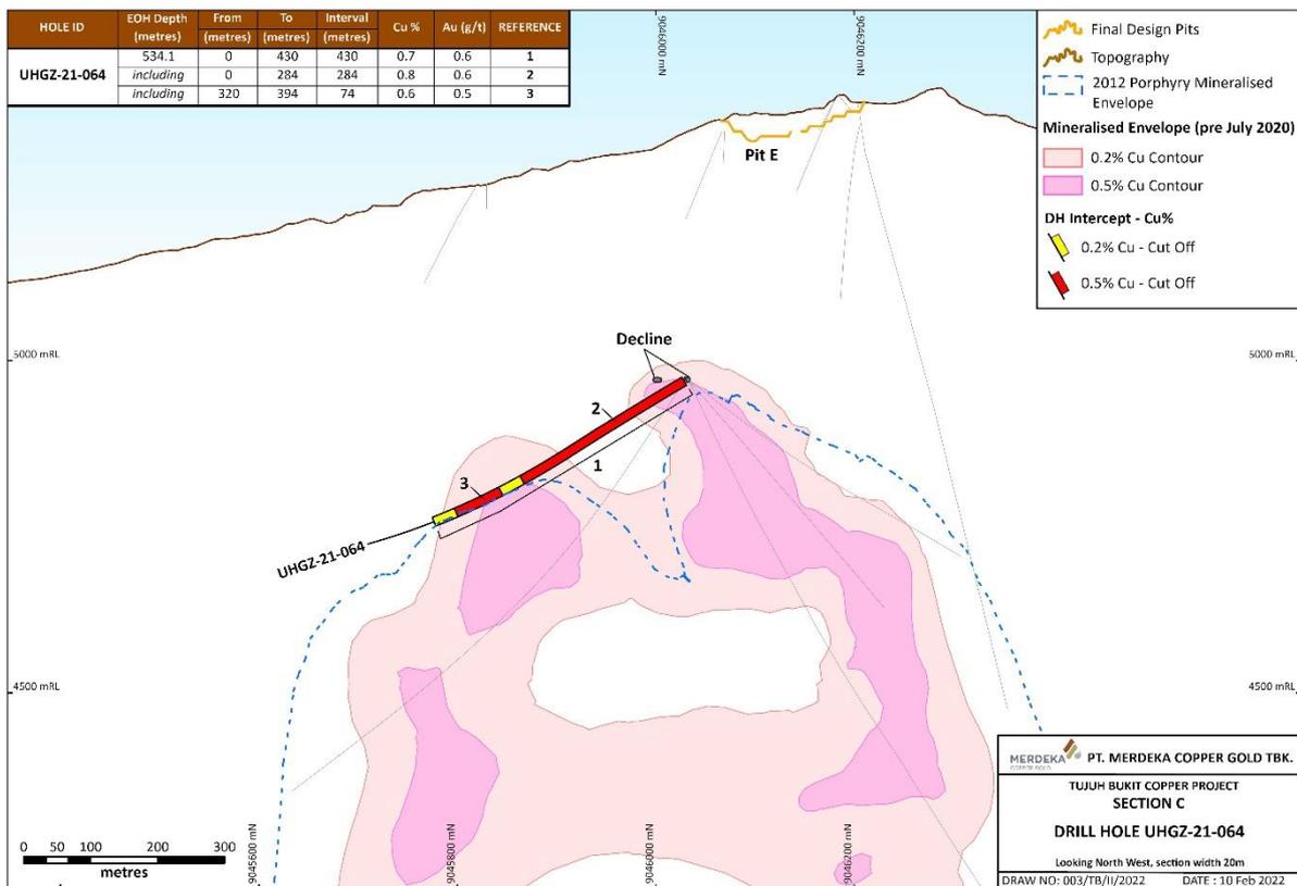
Figure 4: Drill section C, showing drill hole UHGZ-21-064 along with mineralised envelopes and drilling intercept information.
