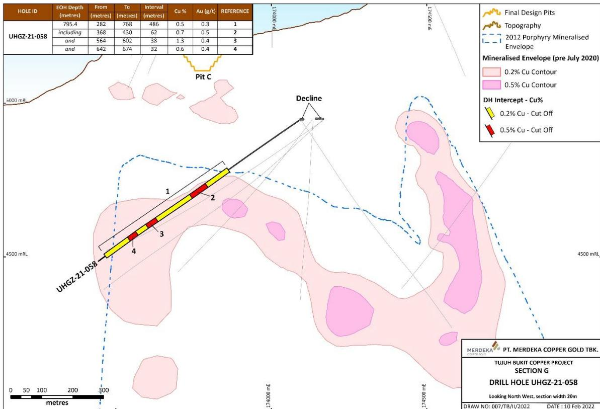
Figure 7: Drill section G, showing drill hole UHGZ-21-058 along with open mineralised envelopes at depth and drilling intercept information.
