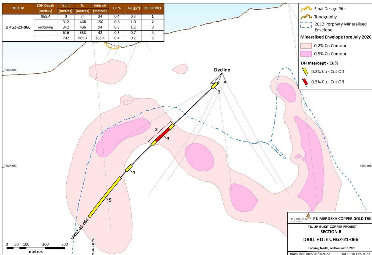
Figure 3: Drill section B, showing drill holes UHGZ-21-066 along with mineralised envelopes and drilling intercept information.
