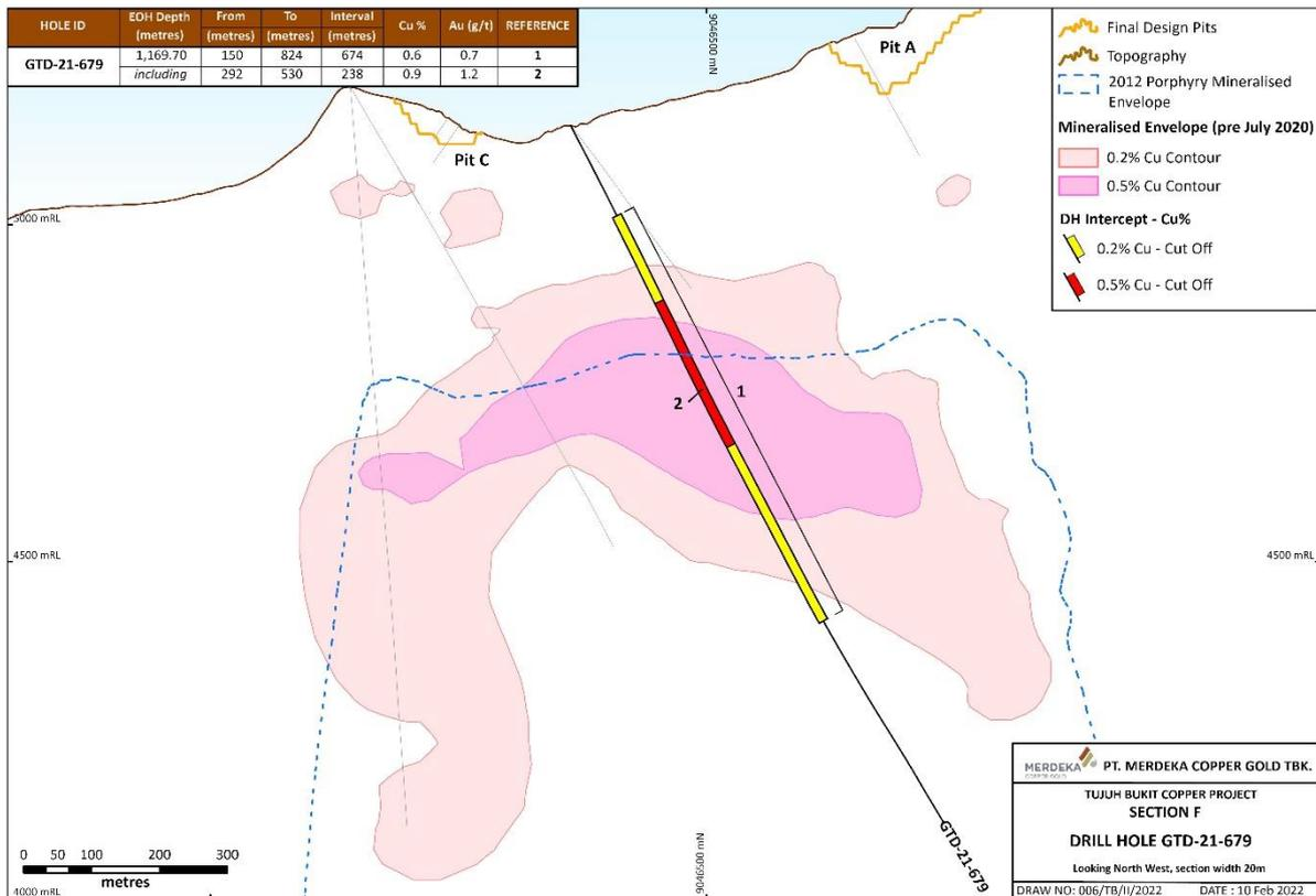
Figure 6: Drill section F, showing drill hole GTD-21-679 along with open mineralised envelopes at depth and drilling intercept information.
