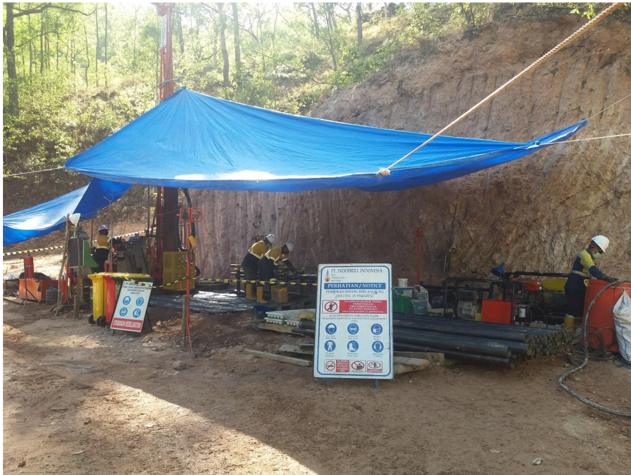
Figure 7: Diamond drilling operations for Regional Exploration to the west of the existing Lerokis pit.
