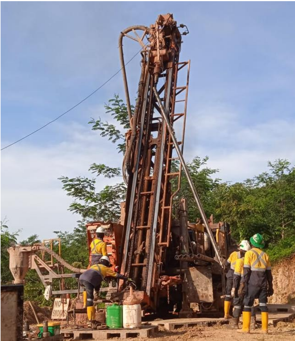
Figure 4: Reverse circulation drilling in Zone D
