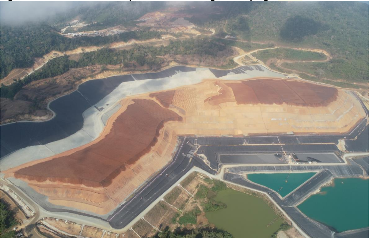
Figure 6 – Aerial view of the Heap Leach Pad showing Lift 5 in progress.
