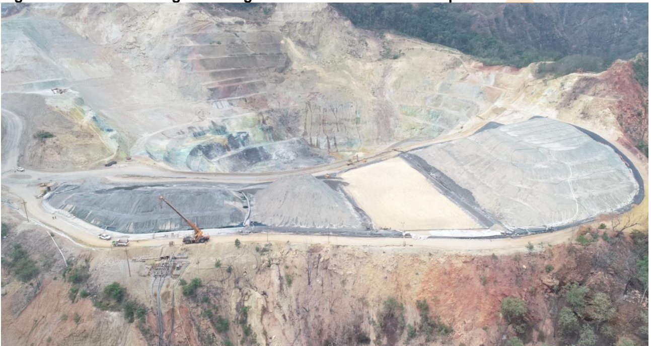
Figure 6 – Photo showing re-mining and extension to the GPLP pads for Lerokis ore.
