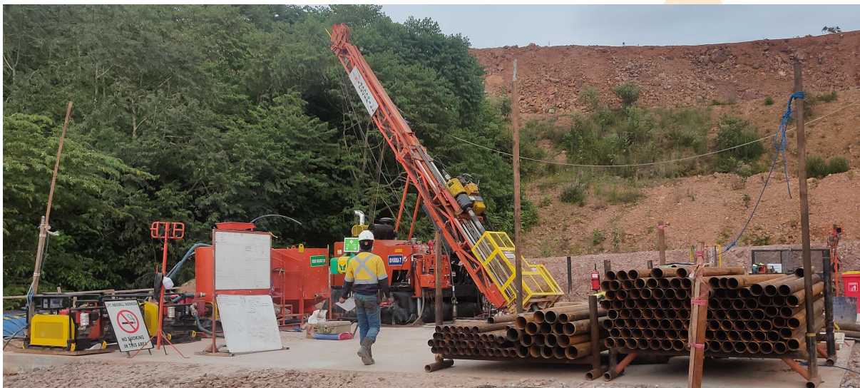
Figure 2: Surface diamond drilling operations at Tujuh Bukit.
