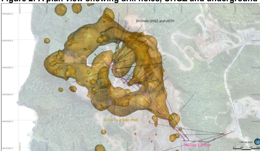
Figure 2: A plan view showing drill holes, UHGZ and underground decline
