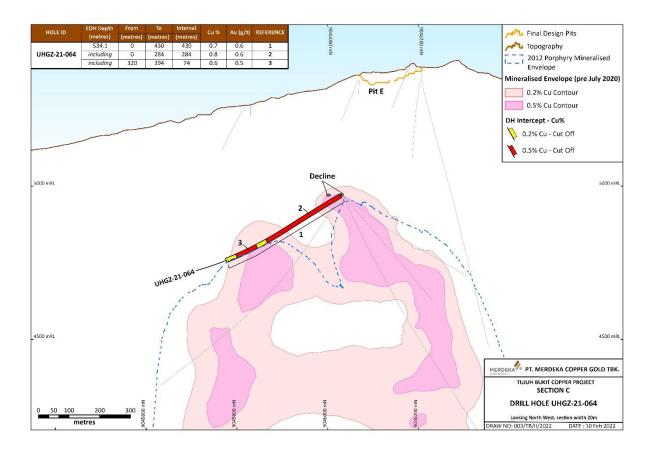
Figure 4: Drill section C, showing drill hole UHGZ-21-064 along with mineralised envelopes and drilling intercept information.
