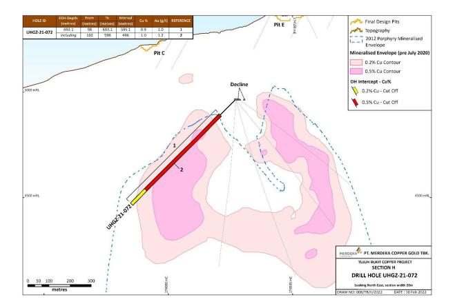
Figure 8: Drill section H, showing drill hole UHGZ-21-072 along with open mineralised envelopes at depth and drilling intercept information.
