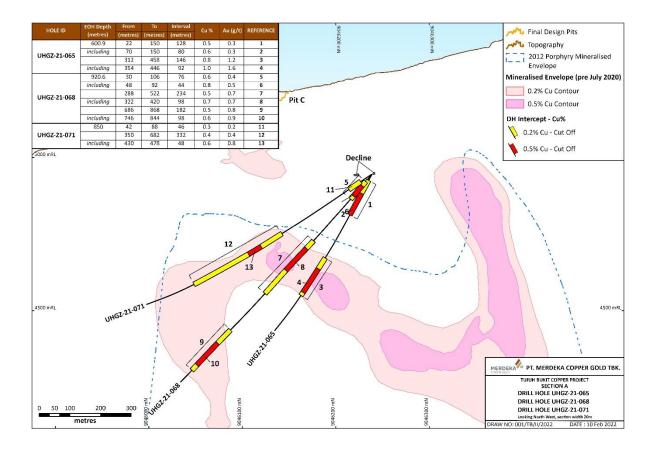
Figure 2: Drill section A, showing drill hole UHGZ-21-065, UHGZ-21-068, and UHGZ-21-071 along with mineralised envelopes and drilling intercept information.
