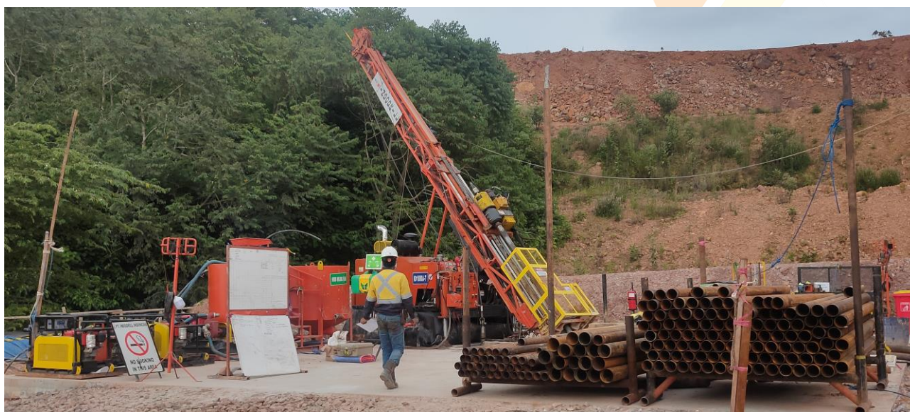
Figure 2: Surface diamond rig setup to commence 1,300 metres Resource Definition drillhole.
