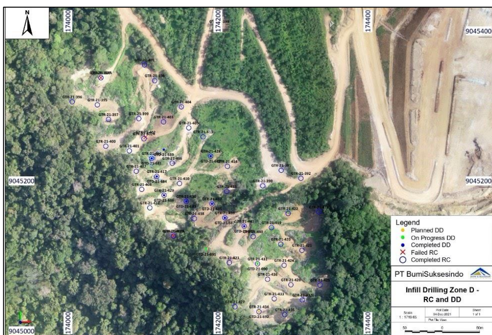
Figure 5: Completed drilling locations in Zone D
