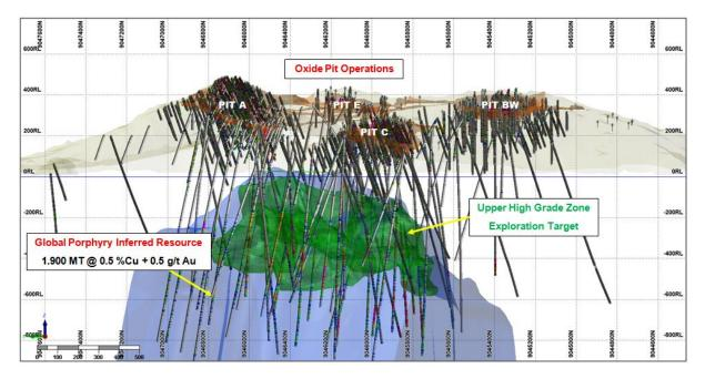
Figure 1: Long section looking due east at the Tujuh Bukit oxide and porphyry deposits<sup>1</sup>
