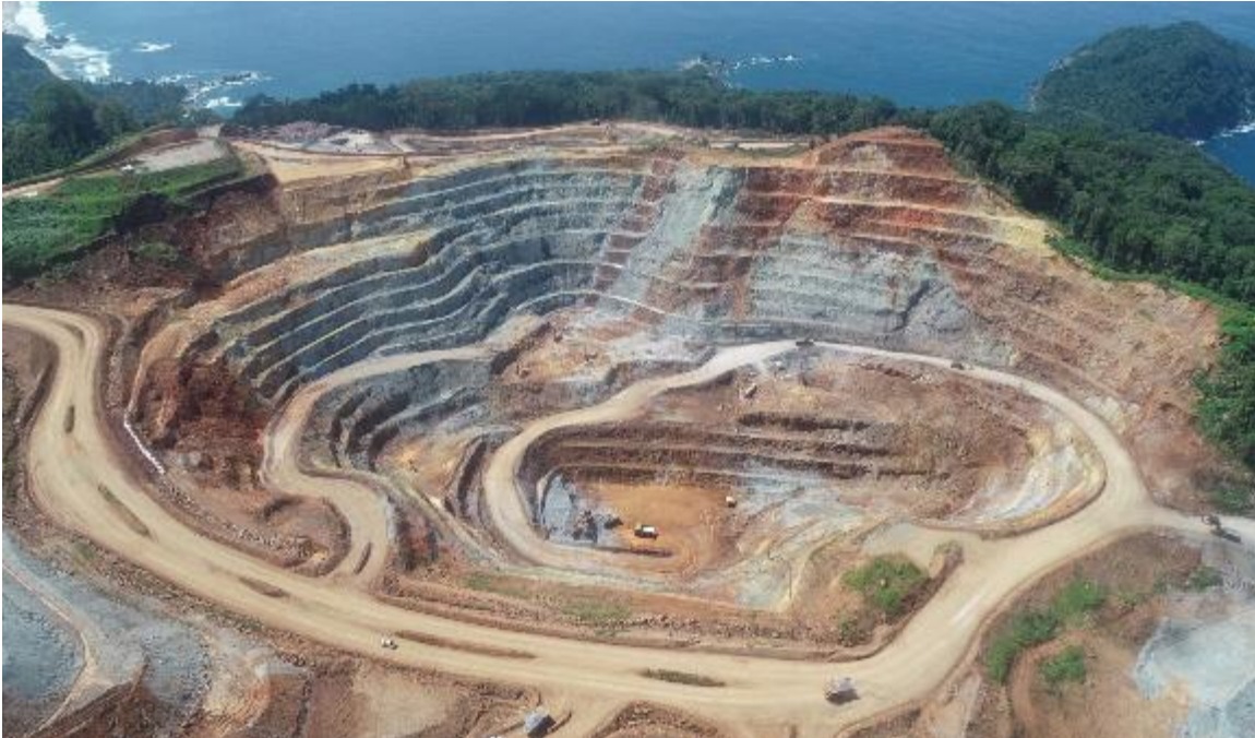
Figure 1 – Open pit mining – Pit B West showing phase 3 in the foreground and phase 4 on left side.
