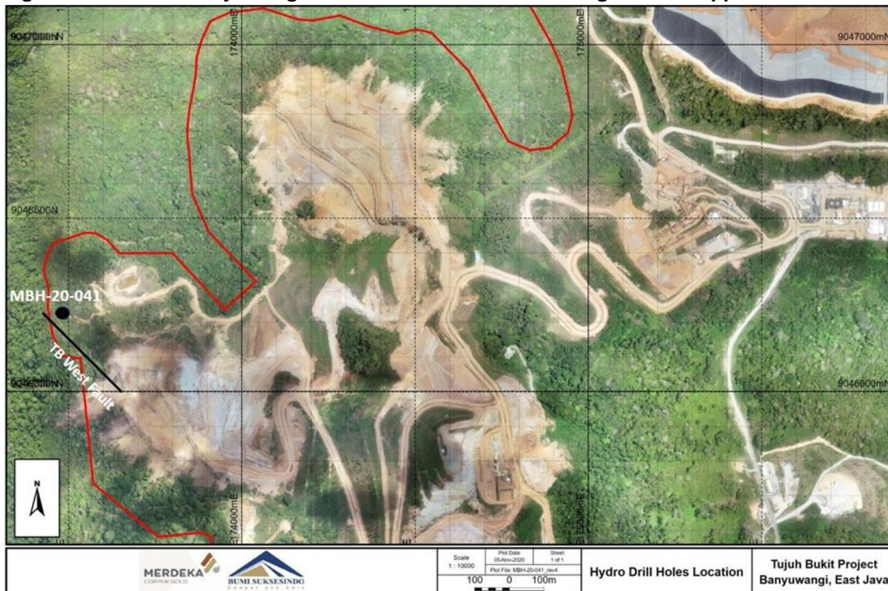
Figure 2: Location of hydrological drill holes near western edge of TB Copper Resource
